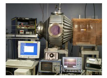
Fig. 2. LAPTAG plasma physics device. The plasma chamber is in the center (the plasma glows with a faint blue light) with the ion acoustic wave launch antenna visible in the right side of the center port. The RF source is enclosed in the screened area and the vacuum system gauges in the rack at the rear. The permanent magnets are held down by the aluminum channels. Magnetic coils are visible surrounding the glass chamber in the plasma source region, but they are not used in these experiments.
