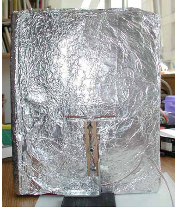
Figure 6: Reflector behind transmitter
